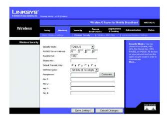
Figure 5-25: Wireless Tab - Wireless Security (RADIUS)
